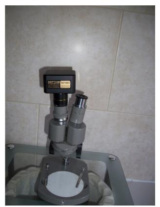
Olympus VA-II stereomicroscope fitted with Swift SC1003 camera Images captured using the Olympus VA-II:
