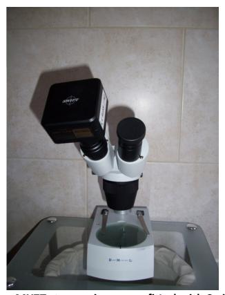
**Brunel Microscopes MX7T stereomicroscope fitted with Swift SC1003 camera**
